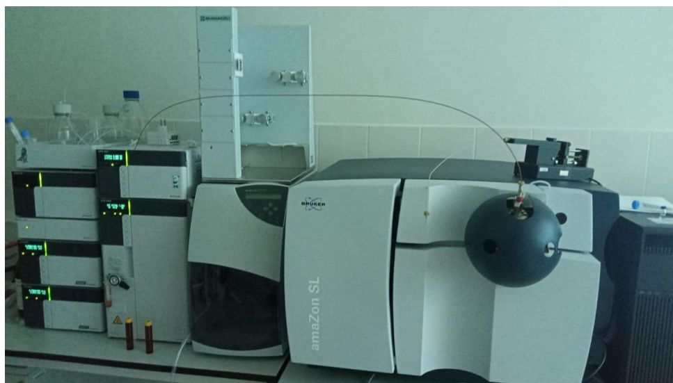
Figure 2. HPLC and ion trap joint system with tandem mass spectrometry
